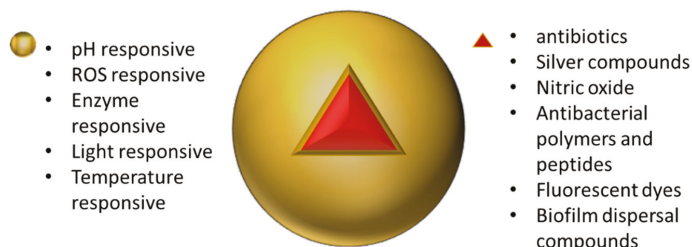
Figure 6. The core-shell architecture of a responsive (nano)material and the possible constituents of the core and shell.
