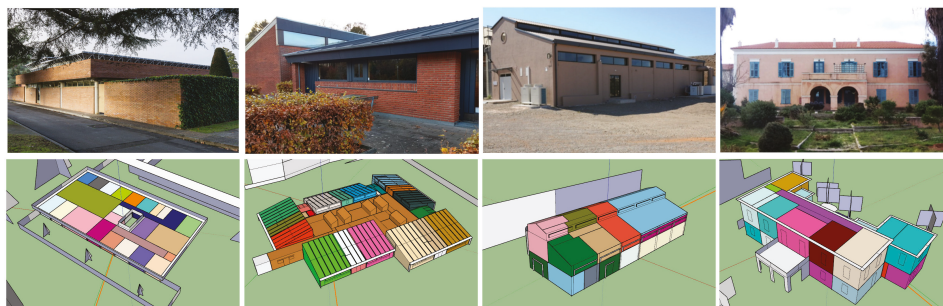
Figure 5. The test sites analyzed. From left to right: office building (University of Navarre, Spain); Gedved school (Denmark); H2SusBuild and administration building in Lavrio (Greece). On top, the real buildings and, on the bottom, the building energy models (SketchUp thermal zone representation, OpenStudio plugin [67]).
