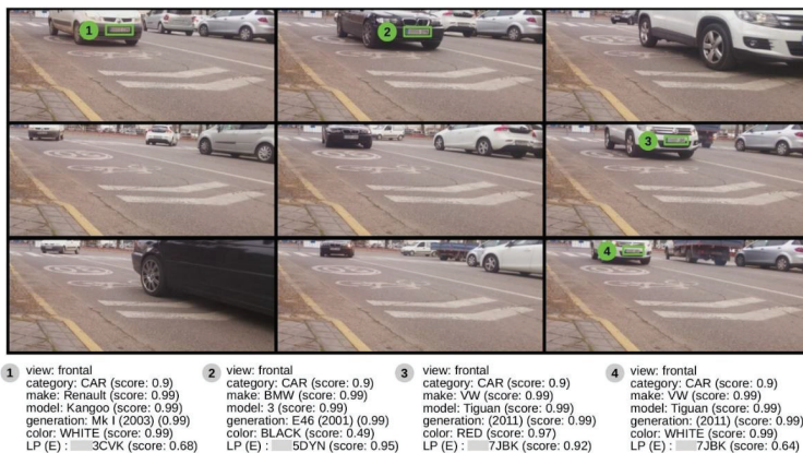
Figure 7. Detection of vehicles in a 3 × 3 image matrix, which allows, by means of a single sending to the cloud, to summarize 9 s of traffic analysis of a given sensor. The system detects both the number plate and certain characteristics of the vehicle, assigning a confidence value to each detection. (To protect personal data, the first three digits of the license plate have been blurred).
