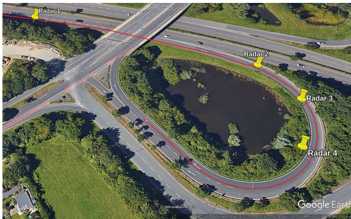
Figure 4. The location of the data recording. Four radar devices were installed at the poles marked here with yellow. The red line shows a path recorded with an RTK-GNSS sensor mounted on a vehicle.
