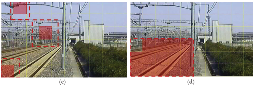
Figure 13. Rough scanning over the scene to find the potential track area. (a) Segmentation result of the whole railway scene images. (b) Different local areas. (c) Scanning the railway scene image roughly using proposed CNN. (d) Area in red dotted rectangle is the potential track area, which will reduce segmentation calculation by three-quarters.
