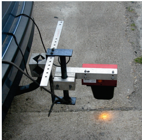
Figure 15. Laser Doppler velocimeter used to generate reference data for the validation of the trajectory reconstruction.
