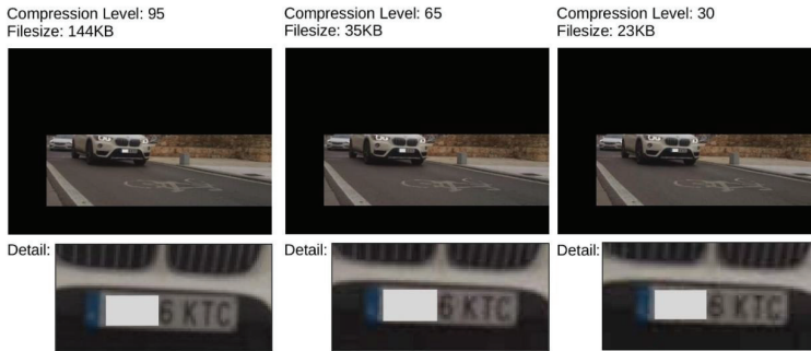
Figure 6. Different compression levels of the JPG standard. With values below 60, with significant loss of high frequency information, the image quality significantly compromises the success rate of the license plate detection algorithms. (To protect personal data, the first three digits of the license plate have been blurred).
