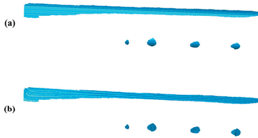
Figure 17. The triangulation of the PCM. (a) The triangle-meshes of the reference PCM; (b) The triangle-meshes of the scratch-surface PCM.
