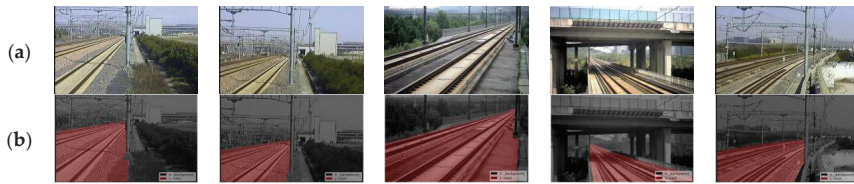
Figure 12. Samples in railway dataset. (a) Images from PTZ cameras under different conditions. (b) Ground truth of the track area.
