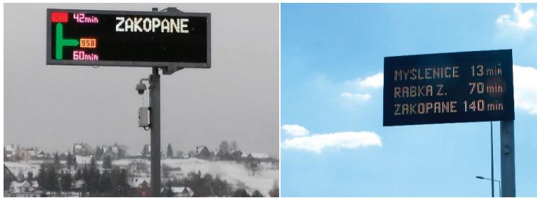
Figure 2. Variable message signs for travel time of the Travel Time Information System (TTIS).
