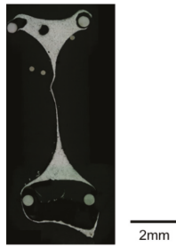
Figure 7. Photomicrograph of cross section of aluminum alloy film (solid fraction f_s = 11\% , holding time t = 0 s).
