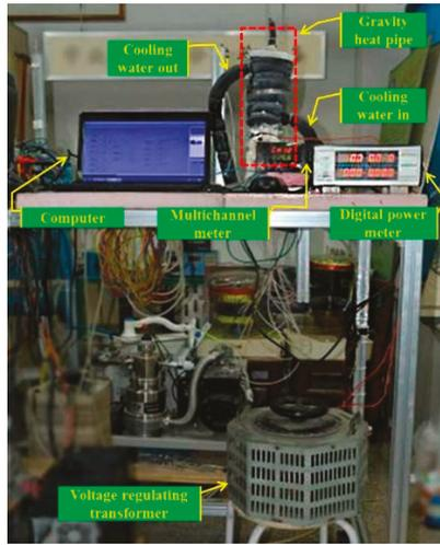
Figure 4. Image of the experimental system.
