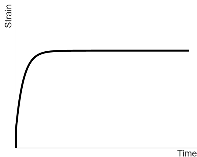
Figure 1. Illustration of creep behavior (increasing strain over time).
