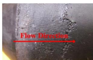
**Figure 1.** Damage of the valve plug results from cavitation erosion [21]-Copyright 2016, Elsevier.
