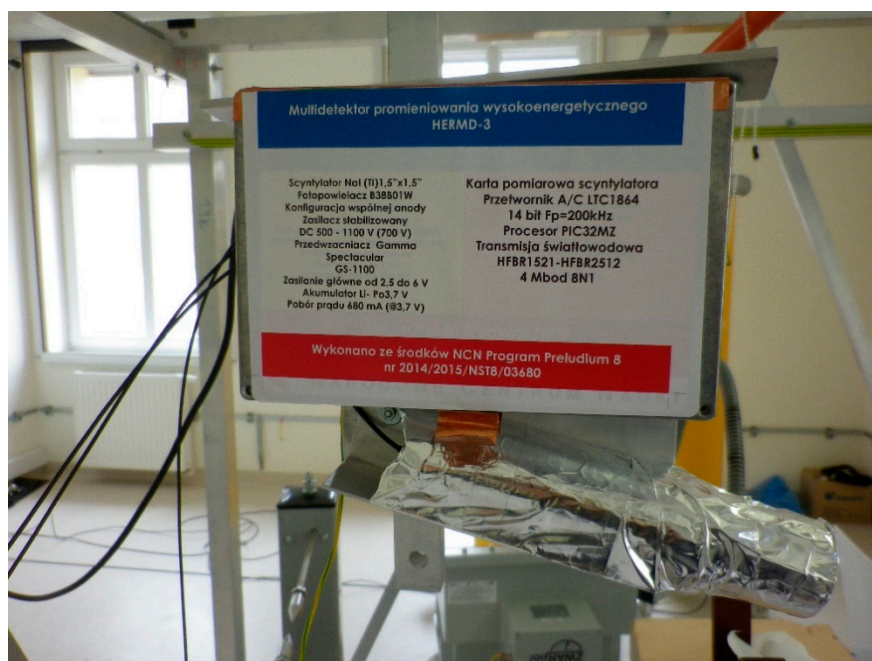
Figure 1. Scintillation detector based on a scintillating crystal, photomultiplier tube, and a measuring card.
