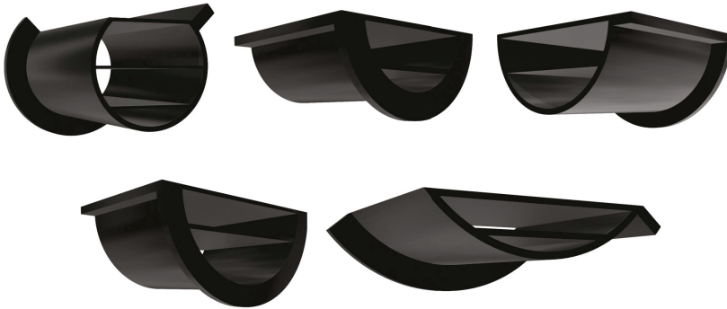
Figure 3. Curved structured used to bend sensor matrix with known curvatures. From left to right, top to bottom, 5, 7, 9, 11, 13 cm.
