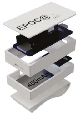
Figure 4. The sensor unit implemented for data logging in the first design stage.
