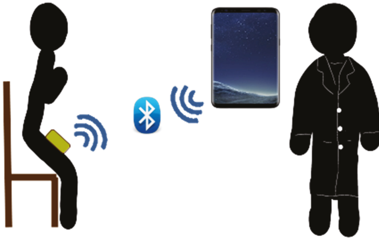
Figure 1. Depiction of the overall experimental setup: The subject stands up from and sits down on a regular rigid chair with the sensing device on one of his thighs; the sensing device is paired with a tablet via Bluetooth; a member of the research team uses the app on board the tablet device to switch the sensor into either calibration or measurement modes, and to visualize the sensor automatic count once the 30-s chair stand test (CST) is over.
