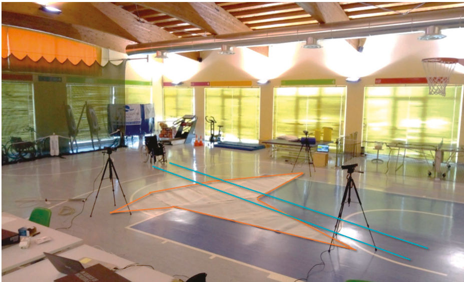
Figure 9. Rehabilitation gym and sensors layout with three-vertex carpet and wheelchair path. This tool allows a faster preparation of the layout of the Mocap system and a reference surface to correctly calibrate the multiple Microsoft Kinect sensors.
