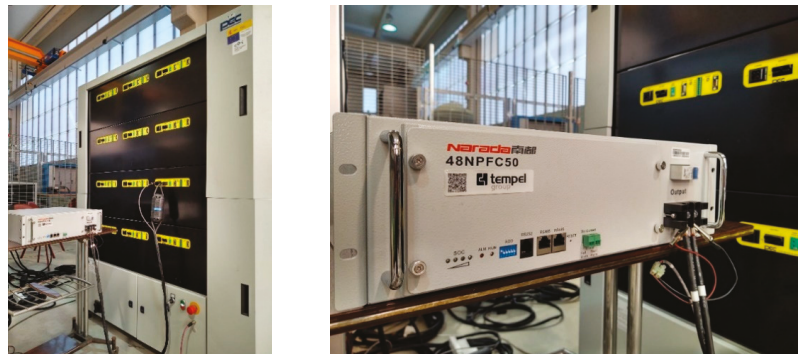
Figure 1. (Left) Laboratory facility for battery testing. (Right) Battery connected to SBT-10050 test equipment.
