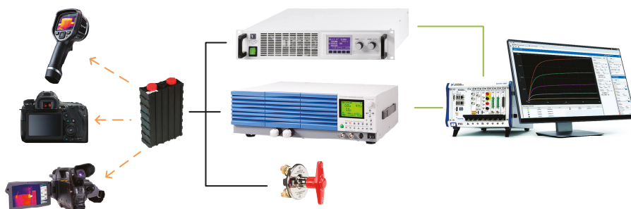
Figure 1. Block diagram of experimental test set-up for selected battery testing.
