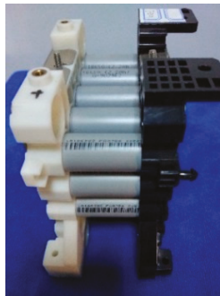
Figure 5. Battery module with 13 cells connected in parallel.
