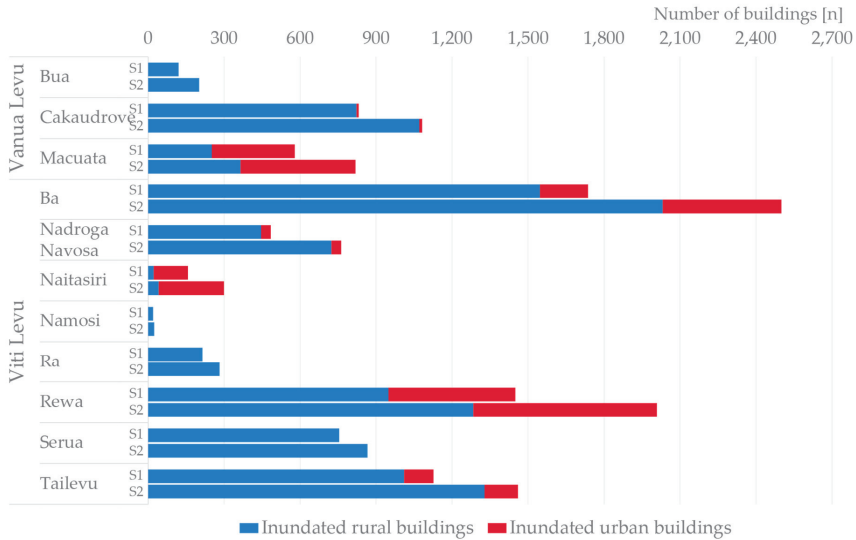
Figure 2. Number of inundated buildings in urban and rural areas of Fiji by province. Scenario 1 refers to projections to 2050 (+ 0.22 m), scenario 2 refers to projections to 2100 (+ 0.63 m).
