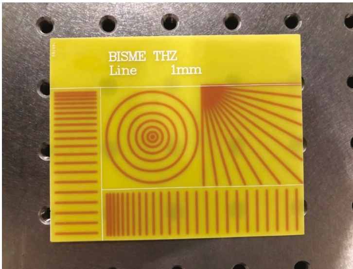
Figure 7. Visual photograph of the resolving power test target.
