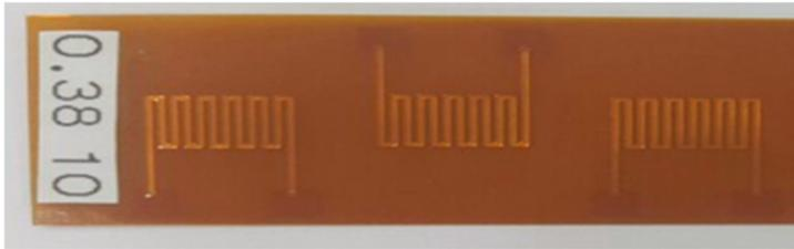
Figure 8. Meander coils with a wavelength of 0.38 mm.
