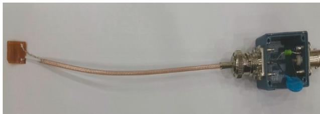
Figure 9. Impedance-matched EMAT transducer.
