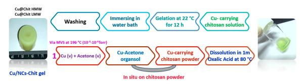
Figure 6. Scheme of preparation of chitosan hydrogels from Cu-carrying chitosan powders.
