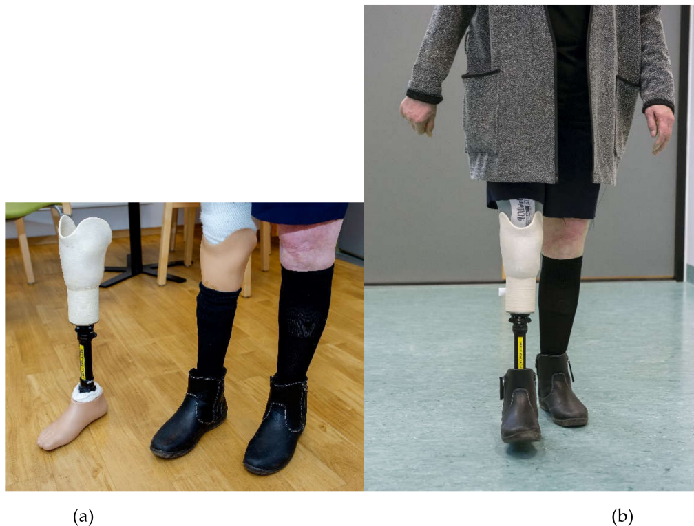
Figure 11. The demonstrator tested by a 70-year-old female with 52 years of experience using a transtibial prosthesis. (a) The patient wearing her conventional prosthesis, with the demonstrator to the left for comparison; (b) The patient walking with the demonstrator.
