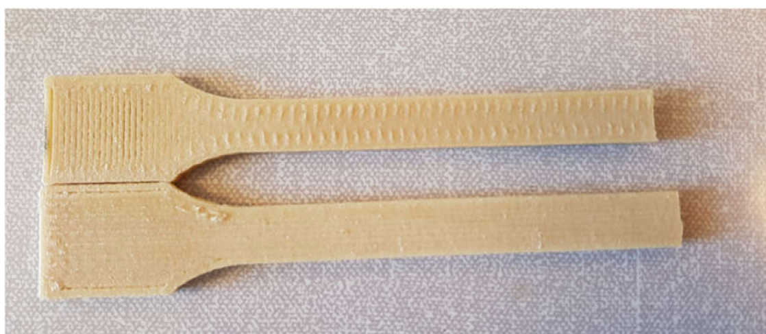
Figure 1. Standard test specimens built with fused deposition modeling (FDM) and with longitudinal lines (bottom) and perpendicular lines (top).
