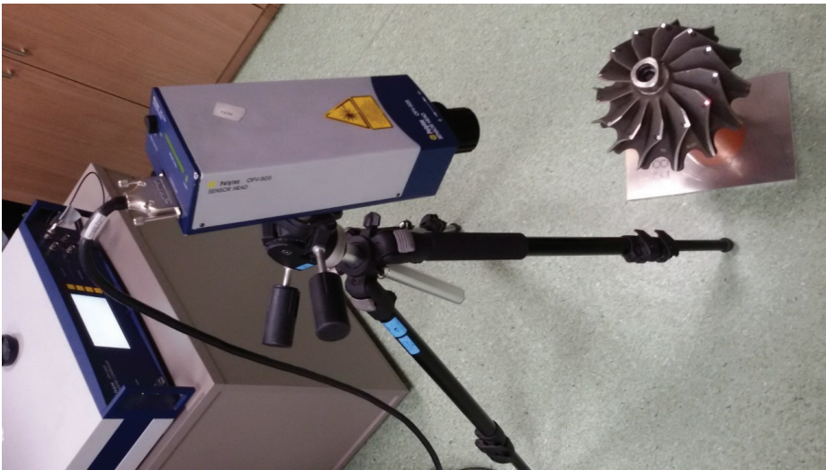
Figure 3. Laser equipment for blade vibration measurement.
