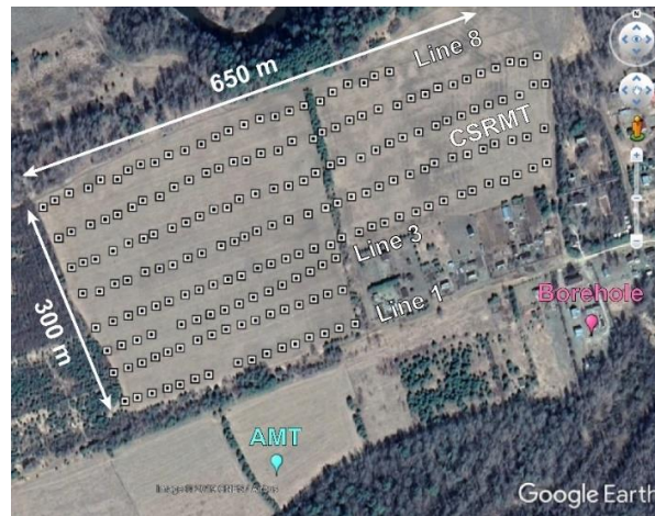
Figure 6. Map of the study area from which the acquisition geometry was taken for the numerical simulation. The boxes depict receiver stations. The receiver lines are numbered from 1 to 8.
