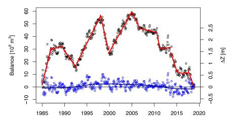
**Figure 4.** Cumulated water balance of Lake H based on raw measurements and a simple correction for long-term trend (**black circles**) and corrected discharges (**blue circles**). Red straight lines indicate manually delineated periods of constant systematic errors, blue line is a local polynomial regression (LOESS) on the corrected discharge. Right axis shows approximate change in storage level.
