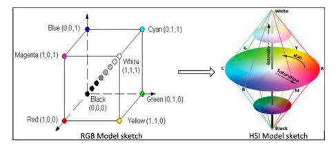
Figure 4. Diagram of the color space model from Red-Green-Blue (RGB) to Hue-Saturation-Intensity (HSI).
