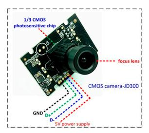
Figure 3. Camera printed circuit board details.
