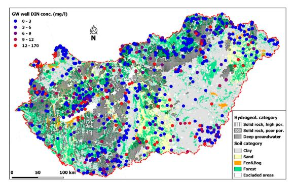
**Figure 3.** Shallow groundwater wells used for model calibration and geological and soil types according to MONERIS classification (GW – Groundwater, DIN – dissolved inorganic nitrogen).
