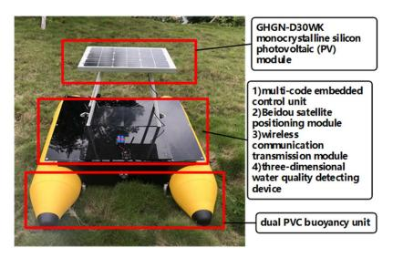
Figure 3. Structural distribution map of the USV. PVC, polyvinyl chloride.
