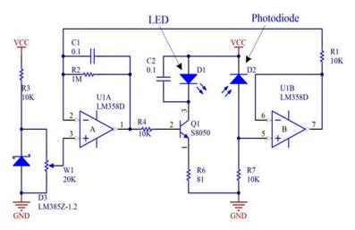
Figure 2. Constant light intensity circuit diagram.
