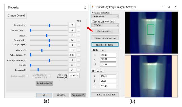
**Figure 5.** Software interface and camera property settings. (**a**) is the camera parameters of this experiment. (**b**) is the main interface of the image processing software.
