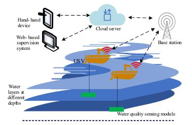
**Figure 1.** The overview of the proposed three-dimensional water quality monitoring system. USV, unmanned surface vehicle.
