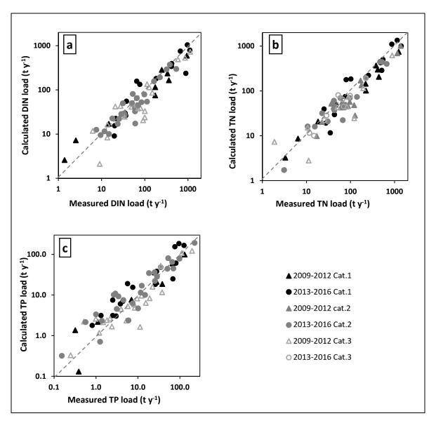
**Figure 7.** Measured and calculated loads at all monitoring stations. (**a**,**b**,**c**) shows the validation results of DIN/TN and TP loads respectively.
