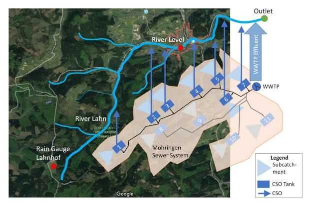
**Figure 1.** Schematic overview of the overlay of the Möhringen sewer system model and the natural baseflow from the river Lahn; CSO = combined sewer overflow; WWTP = wastewater treatment plant; grey sewer system structures were not considered in the model. (Source: Google Maps)
