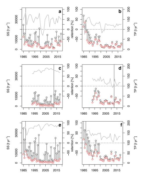
**Figure 5.** Fluxes (black circles: incoming, red circles: outgoing, connected for clarity) and retentions (gray line) of suspended solids (SS) and total phosphorus (TP) in Lake H (**a**,**b**), in the area of phase 2 (**c**,**d**), and in the entire system (**e**,**f**). In c and d, the vertical line indicates diversion of flow from the Ingói Reeds to Lake F in January 2013.
