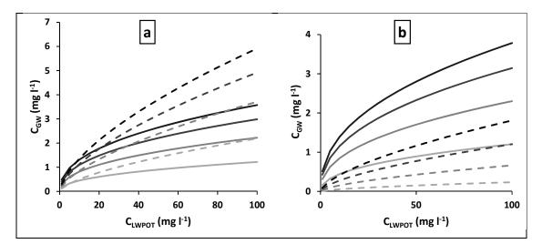
**Figure 8.** Groundwater nitrogen concentration vs. potential leachate concentration and their dependency of annual recharge using old and new retention parameters. (**a**) Consolidated rocks with high porosity; (**b**) unconsolidated rock with shallow groundwater. Dashed line: original parameters; continuous: adjusted parameters. Recharge values 10, 20, 30, 40 mm  $y^{-1}$  from lighter to darker colors.
