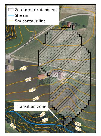
**Figure 1.** Example of a zero-order catchment (catchment area belonging to a single overland-channel transition zone) based on a DEM with  $10 \times 10$  m resolution and the D8 single flow direction algorithm [41].
