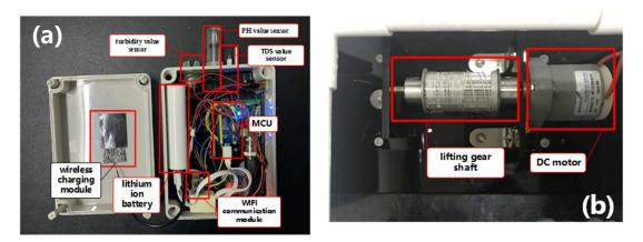
Figure 6. (a) Arrangement of sensors of water quality monitoring system (WQMM), (b) Lifting device.
