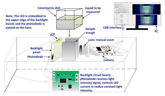
Figure 1. Structure of a water chromaticity measurement system.
