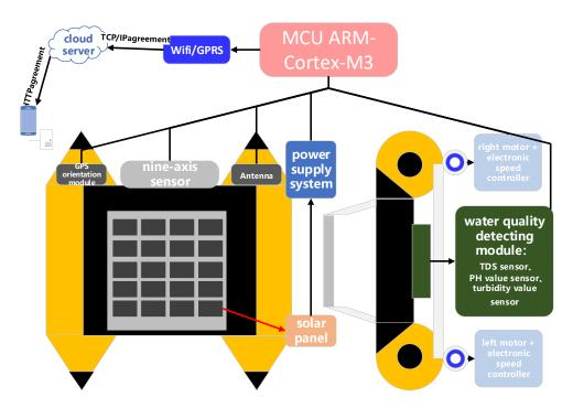
**Figure 2.** The overall architecture design of the unmanned service vehicle (USV). GPRS, general packet radio service; MCU, micro control unit; GPS, global position system; TDS, total dissolved solids; ARM, advanced reduced instruction-set computer machine.
