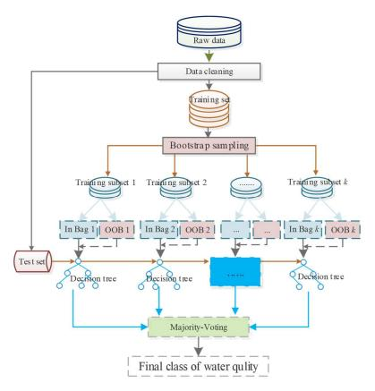
Figure 8. Flowchart of the water quality analysis algorithm. k, the number of trees; OOB, out-of-bag.
