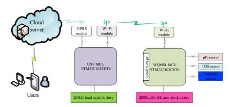
Figure 7. Diagram of the data transmission process. WQMM, water quality monitoring module.
