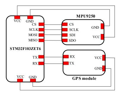
**Figure 4.** The architecture of the automatic positioning cruise system. GPS, global positioning system; VCC, volt current condenser; GND, ground; TX, transport; RX, receive; CS, chip select; SCLK, serial clock; MOSI, master out slave in; MISO, master in slave out; SDI, serial data input; SDO, serial data output.
