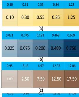
**Figure 15.** Measurement results of standard solution for ammonia nitrogen, phosphate, and chloride. (a) is the measurement results of standard solution for ammonia nitrogen. (b) is the measurement results of standard solution for phosphate. (c) is the measurement results of standard solution for chloride.
