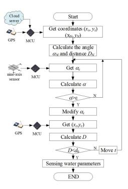
**Figure 5.** Flowchart of the APCS. ( $x_s$ ,  $y_s$ ), the starting position; ( $x_N$ ,  $y_N$ ), the next position;  $D_N$ , the distance between the next and starting positions;  $\alpha_N$ , the angle between the next and starting positions;  $\alpha_C$ , the current heading angle;  $\alpha$ , the angle deviation; $\varepsilon$ , the angle resolution; ( $x_C$ ,  $y_C$ ), the current position; D, the distance deviation;  $d_0$ , the distance resolution; t, moving time.
