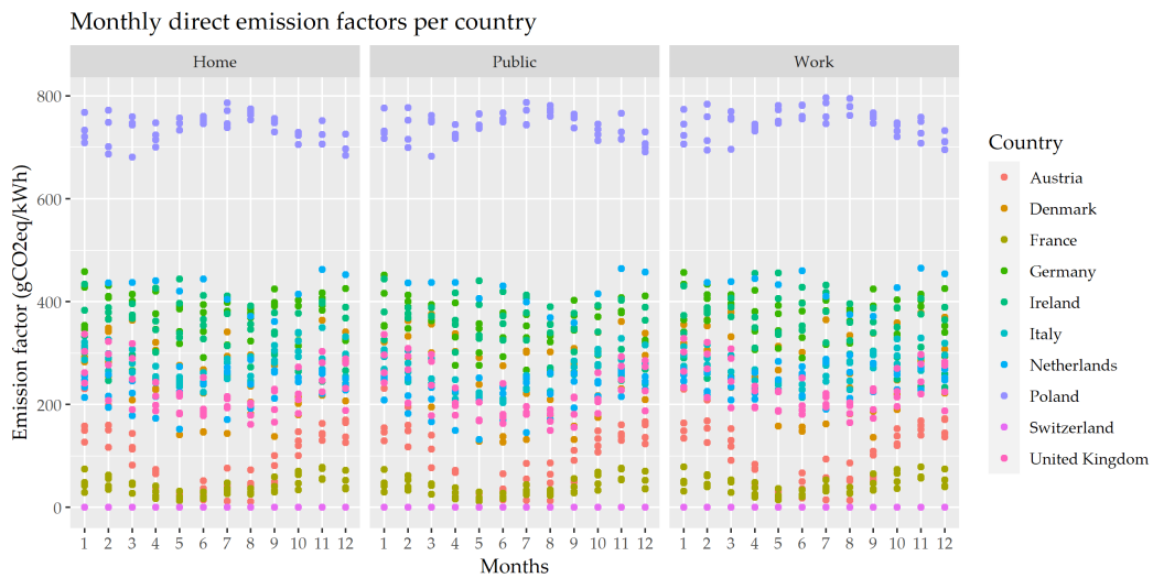
Figure 6. Monthly emission factors of EV charging in each country and each month.
