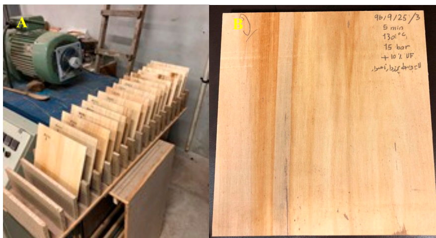
Figure 1. Panels produced and trimmed, ready to be cut to size for each test according to the relevant standard (A); front surface of a trimmed plywood panel (B).
