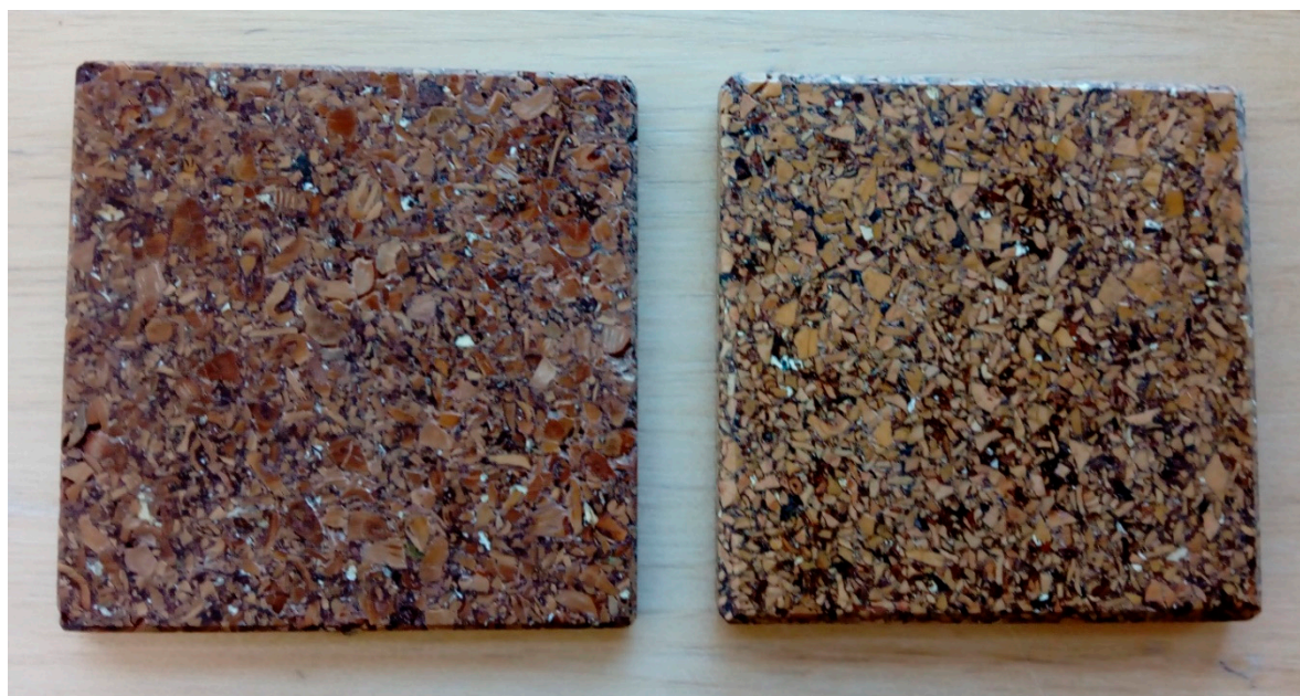
Figure 1. Hazelnut and walnut 10 mm thick samples bonded with PUR; 1000 kg/m 3 density; composition: 70% fine-grained particles (<3 mm) and 30% coarse-grained particles (3–6 mm).
