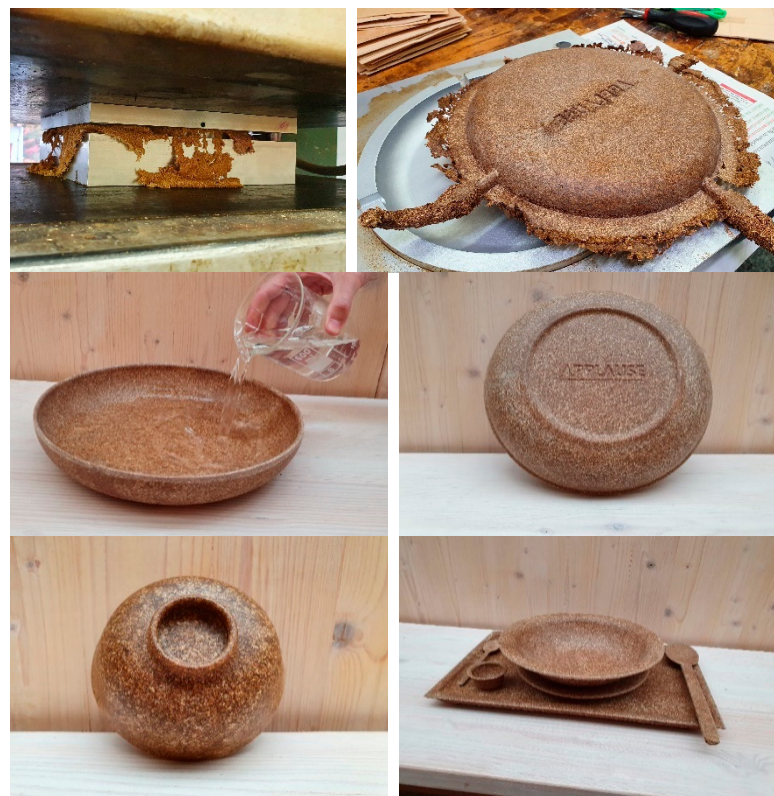
Figure 15. Some examples of 3-dimensional shaped WPC products made from invasive alien woody plants.
