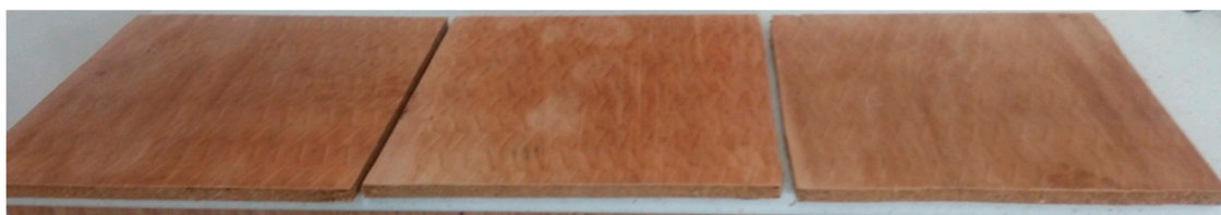
Figure 1. Eco-friendly panels from industrial waste fibres bonded with magnesium lignosulfonate and veneered with beech veneers; 720 \text{ kg}\cdot\text{m}^{-3} target density, 18 mm thickness and 15% lignosulfonate content.
