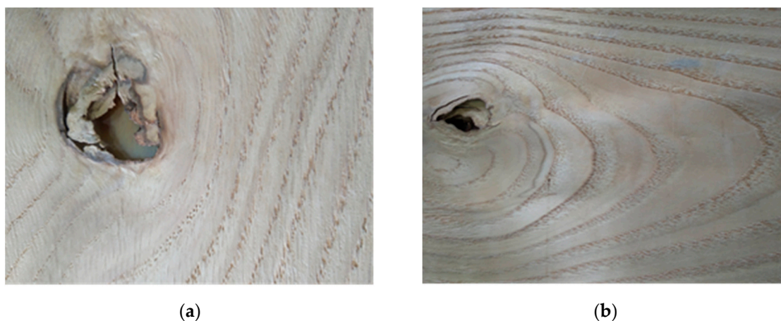
Figure 1. Dead knots in oak wood sliced plain-cut veneer (a), and in chestnut wood sliced veneer (b).
