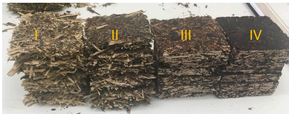
Figure 7. Particleboard samples containing 4.7%, 9.1%, 20%, and 33.3% (I–IV in order) partially liquefied bark without using MUF adhesives.
