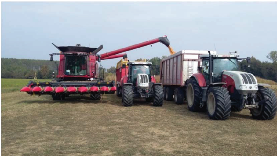
Figure 3. Simultaneous unloading phase of Maize kernel and cob tanks using Harcob system.
