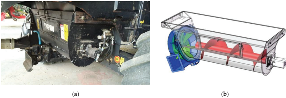
Figure 2. (a) Thievin system “Turbopaille” for chaff collection and (b) schematic representation.
