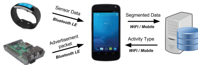
Figure 1. Overall system architecture.
