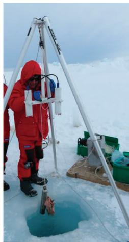
**Figure 2.** Essential structure of the mini-BRUV system. The prototype was deployed through ice holes of about 40 cm diameter.
