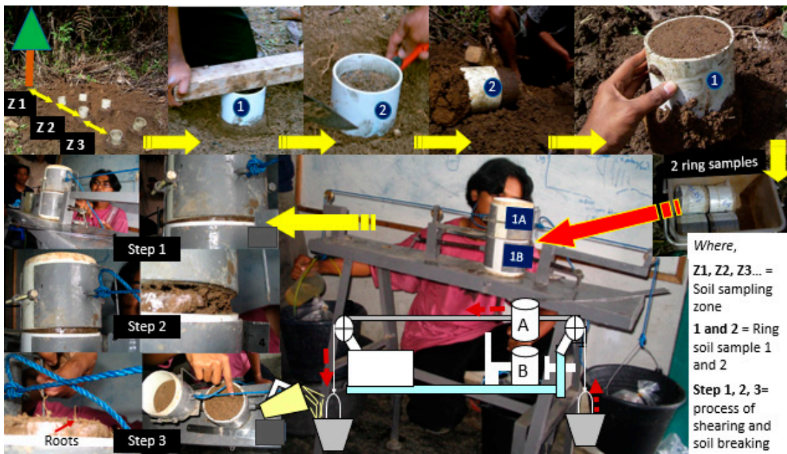
Figure 2. Taking soil samples in the study site in a double ring and measuring soil shear resistance by increasing the pull by adding water to a bucket until the upper ring moves.
