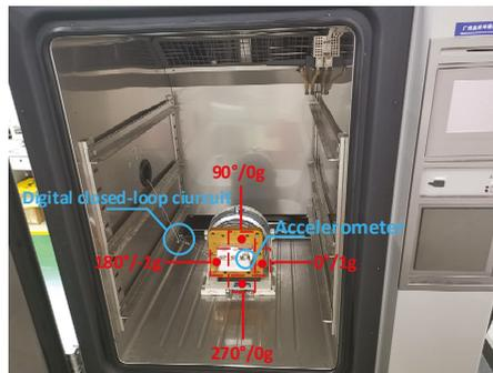
**Figure 4.** QFA assembled on an index head in temperature-controlled oven, and the index head can be controlled by oven to rotate. The inputs to QFA at  $0^{\circ}$ ,  $90^{\circ}$ ,  $180^{\circ}$ ,  $270^{\circ}$  are  $1\text{ g}$ ,  $0\text{ g}$ ,  $-1\text{ g}$ ,  $0\text{ g}$ .
