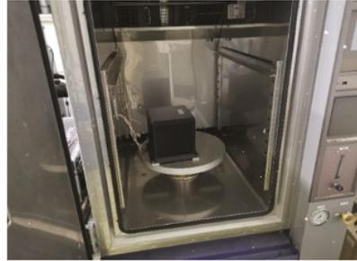
Figure 8. INS in temperature-controlled oven.
