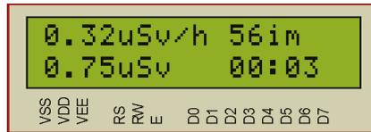
Figure 9. Simulation of the system operation in dosimeter mode.
