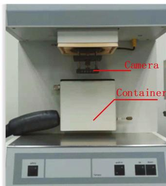
**Figure 2.** The equipment of creep experiment mainly consists of two parts, a high-resolution camera and a container. Camera can record the micro deformation of object in the container, and the container is a temperature-controlled oven which can provide precise temperature from  $-70\text{ }^{\circ}\text{C}$  to  $+100\text{ }^{\circ}\text{C}$ .
