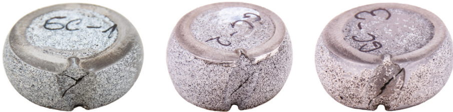
Figure 14. Notched cylinder specimens after testing with fractures in the notch region.
