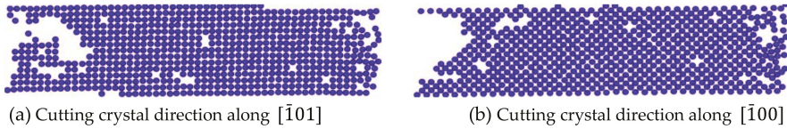
Figure 11. Atomic distribution of machined surface under different cutting crystals.
