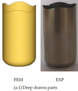
Figure 12. Comparison of cup wall thickness between conventional and MDR die applications obtained by FEM simulation (DR: 2.25; initial blank diameter: 90 mm). (a) Conventional die (Radius 3.5 mm); (b) Multi draw radius die type I (Radius 3.5–7 mm).
