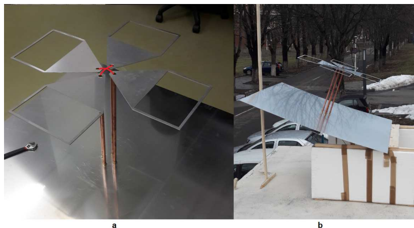
Figure 3. The antenna prototype: feeder (a) and a caption during measurements (b). The position of the feeding inner conductor of the coaxial cable is illustrated with red (a). The inner conductor is soldered on one blade and the outer conductor on the other, similar to [12] © 2012 IEEE.
