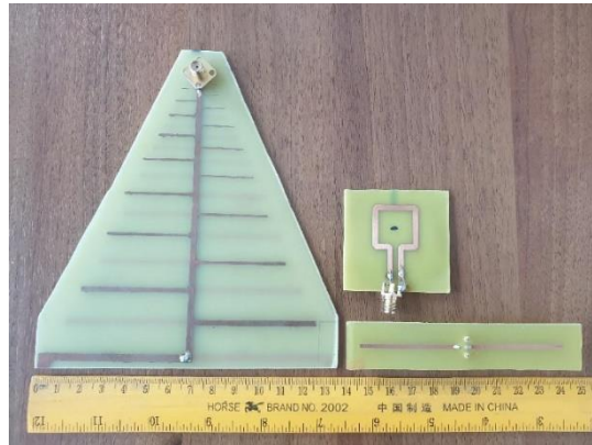
Figure 10. Antennas under test and probe antenna.
