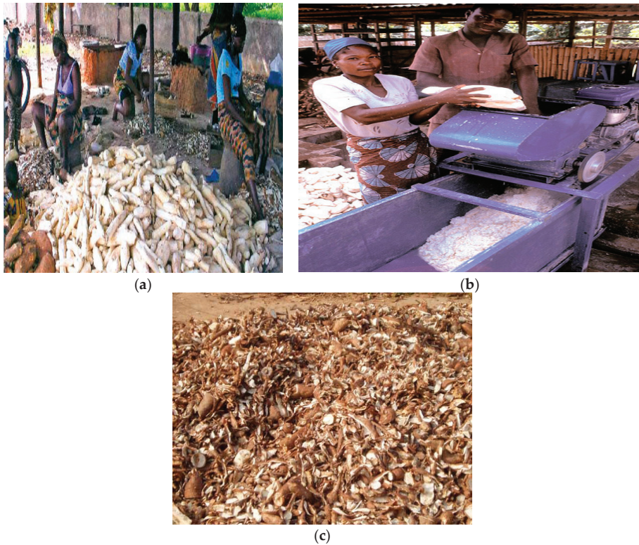
Figure 3. Activities in the Cassava Processing Factory. (a) Cassava peeling section; (b) Cassava grinding machine in operation; (c) Cassava peel dump site.
