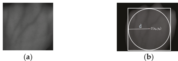
Figure 3. Captures the region of interest (ROI) area. (a) Maximum inscribed circle; (b) ROI area.
