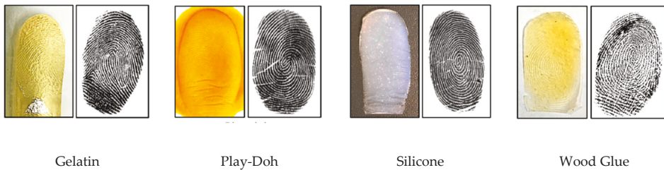
Figure 1. Examples of fingerprint artefacts fabricated using different materials. A real image of a fabricated fingerprint is shown on the left and a scanned image using a fingerprint sensor is shown on the right [4].
