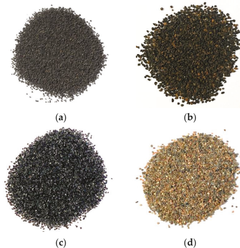
Figure 1. (a) Filtralite Pure HC 0.5–1, (b) Filtralite Pure NC 1.5–2.5, (c) anthracite 0.8–1.6 mm, (d) sand 1.2–2.0 mm “Rådasand”.
