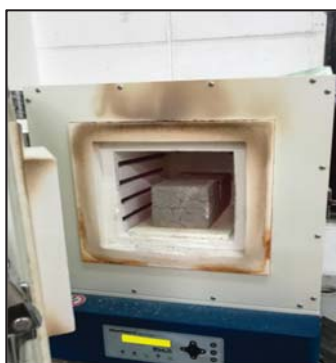
Figure 1. Overview of an automatic electrical furnace.
