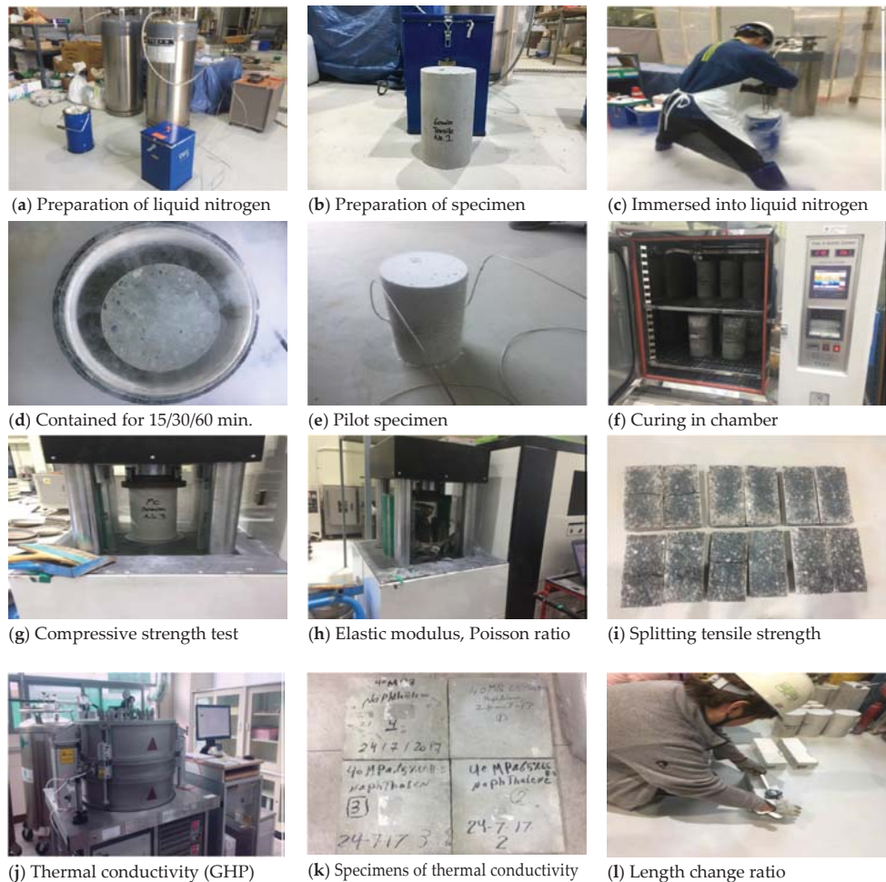
Figure 3. Test A method under cryogenic condition.
