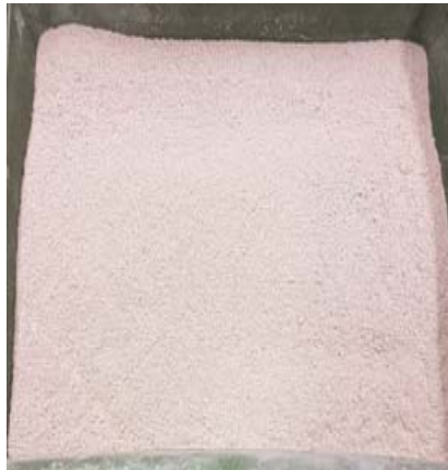
Figure 2. Recycled cement mortar (fine fraction) obtained after thermal and mechanical treatment, used to tests.
