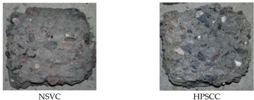
Figure 6. The cleaned core of broken cubes heated to 700 °C.
