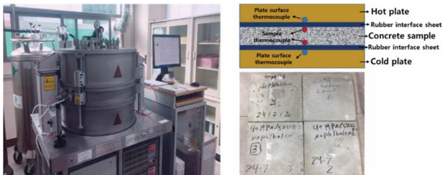
Figure 10. GHP (Guarded Hot Plate) 456 Titan and set-up of the sample, thermal sensors and plate.
