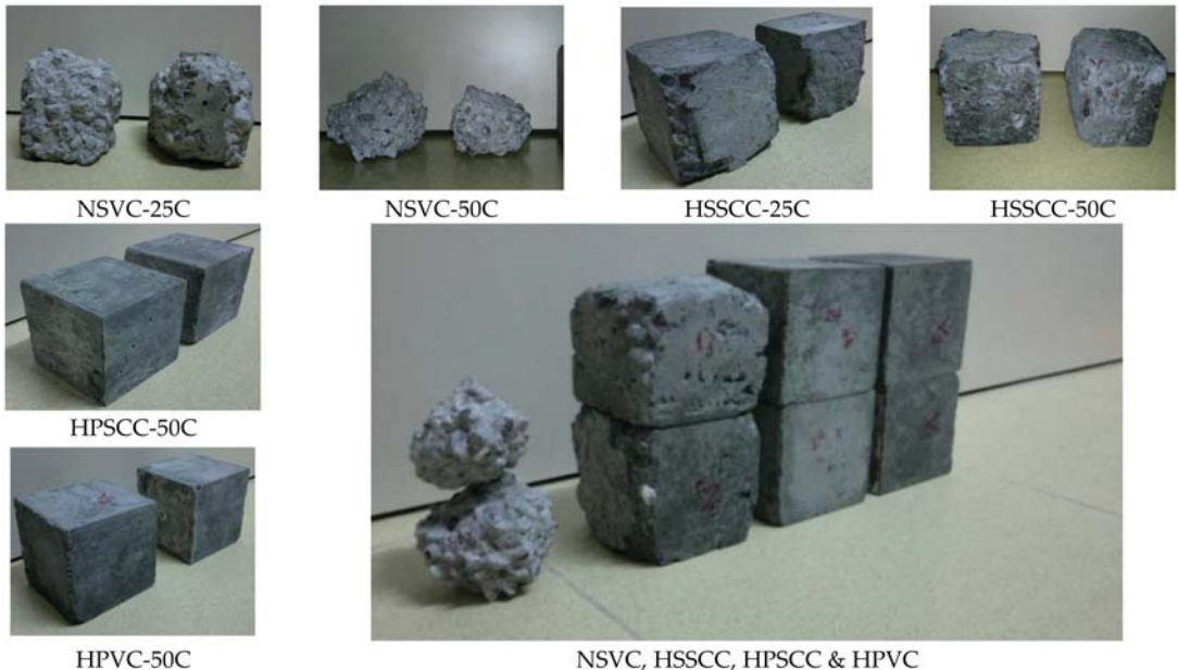
Figure 7. Freeze-thaw specimens after 25 and 50 cycles for NSVC and HSSCC and 50 cycles for HPSCC and HPVC.
