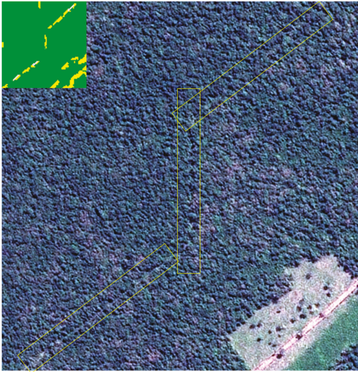
Figure 12. Location of canals hardly visible in SPOT-6/7 corresponding with the detections by Sentinel-1 in the black ellipse of Figure 11b. The inset located in the upper-left shows the corresponding area of the Sentinel-1 NRT canal gap map.
