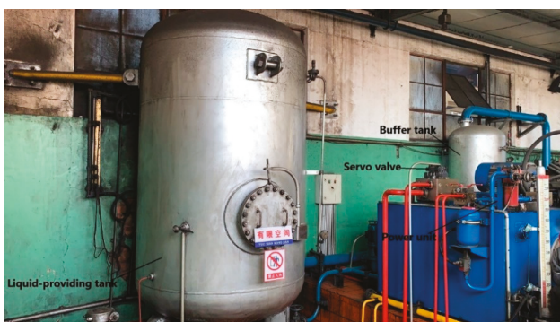
Figure 5. Photograph of the energy-saving buffering system.
