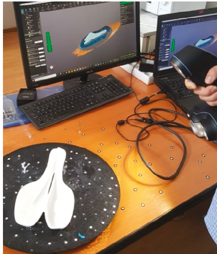
Figure 11. Positioning of the bike saddle on the rotary table of the scanning system
