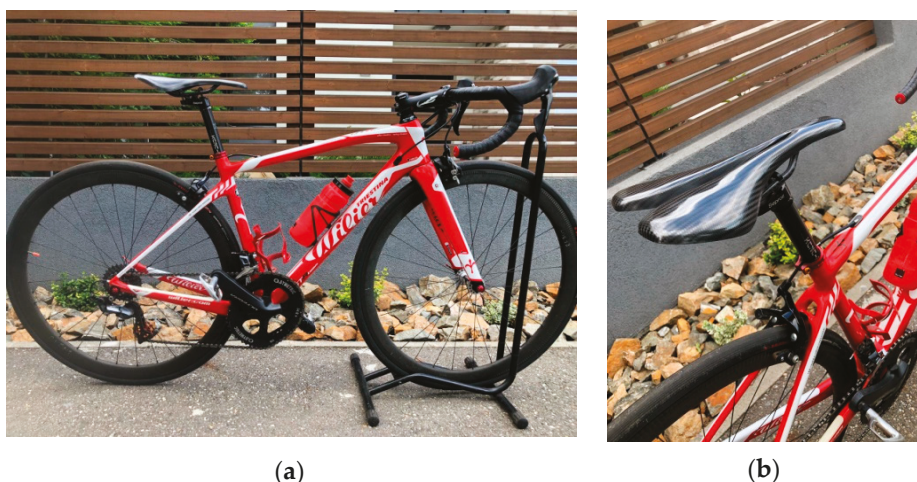
Figure 15. The CFRP saddle prototype assembled on a road bike: (a) view about the bicycle; (b) detail of the saddle.
