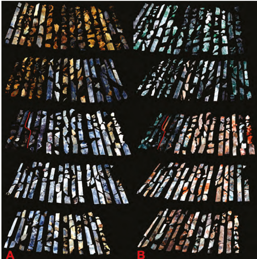
Figure 4. (A) True-color image of the core samples; and (B) false-color composite of bands 206-217-228 in the short wave infrared (SWIR) data of the core samples. Pixels other than the core samples have been masked out. The RGB bands in (B) have wavelengths of 2203, 2271, and 2340 nm, respectively. The red lines show the interpreted unconformity between the basal Claron Formation and the underlying Callville Limestone.
