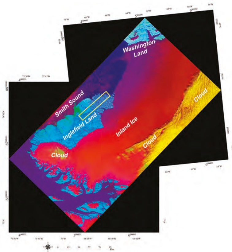
Figure 4. A regional view of the northwestern part of Greenland generated using a mosaic of Landsat-8 images as RGB false-color composite of the normalized difference snow index (NDSI), Al-OH-bearing alteration minerals index (Al-OH-MI), and thermal radiance lithology index (TRLI). Yellow rectangle shows the location of the Cu-Au mineralization belt.
