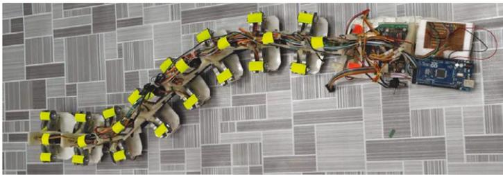
**Figure 1.** The snake robot with markers on the dorsal side.
