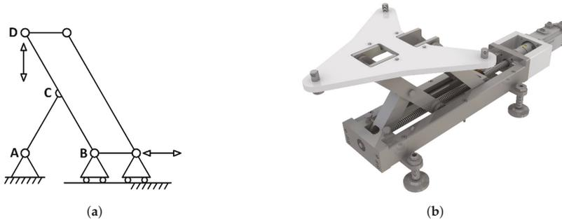
**Figure 16.** Lifting system. (a) lifting system scheme; (b) lifting system assembly.
