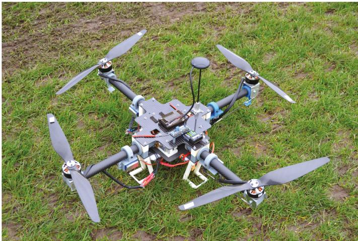
Figure 14. Dual-tilting quadcopter prototype.
