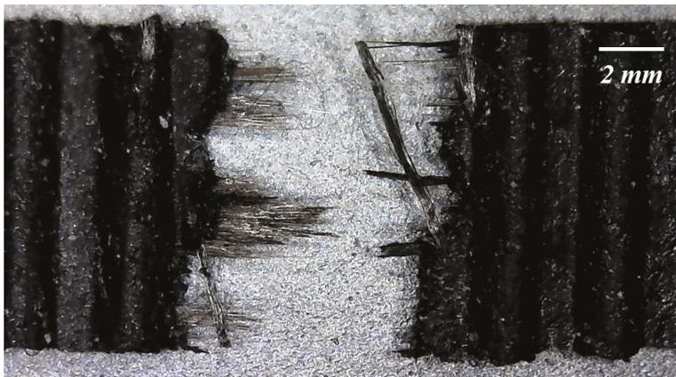
**Figure 3.** Belt break interface, showing broken fibers.
