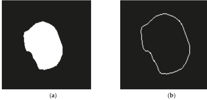
Figure 4. (a) Binary image, (b) border extraction.
