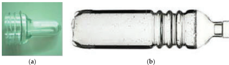
Figure 2. (a) Preform in PET (polyethylene terephthalate), from which the bottle is obtained through a thermoforming process; (b) example of the final geometric complexity of a bottle.
