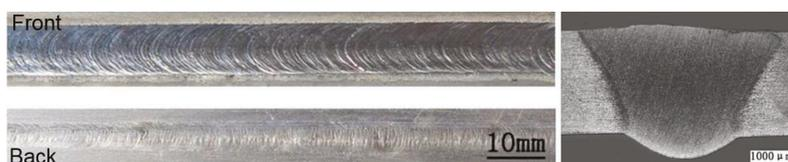
**Figure 4.** Appearance and the macrostructure of hybrid welding Al alloys joint.
