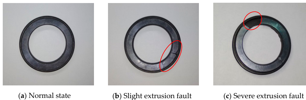
Figure 3. Rotating ring in different extrusion fault.
