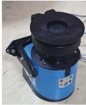
Figure 6. SICK (Sick AG company, Germany) laser range finder (LMS100-10000).
