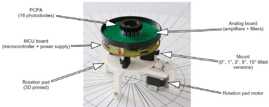
Figure 6. Photo of the PCPA deployed on the turntable, used in the automatic measurements.
