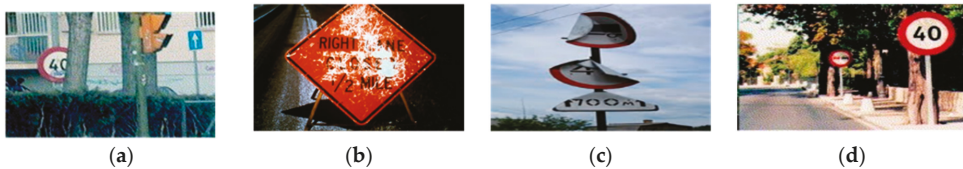
Figure 1. Non-identical traffic signs: (a) Partially occluded traffic sign, (b) faded traffic sign, (c) damaged traffic sign, (d) multiple traffic signs appearing at a time.
