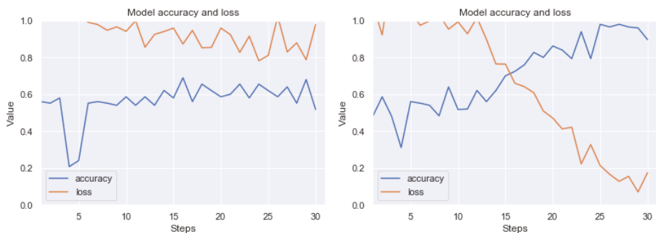
Figure 19. Exemplary learning effect before (left side) and after using our technique (right side). Result for MOSCOW dataset. Class 0 (without artefacts) vs. class I (with weak artefacts) vs. class II (with strong artefacts). The line graphs shows accuracy (blue) and loss (orange) for 15 epochs (30 steps from batch). Although the image dataset is relatively small for CNN, there can be observed a good trend in increasing accuracy, while minimizing loss.
