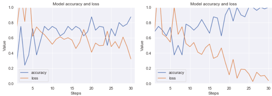
Figure 18. Exemplary learning effect before (left side) and after using our technique (right side). Result for MOSCOW dataset. Class 0 (without artefacts) vs. class II (with strong artefacts). The line graphs shows accuracy (blue) and loss (orange) for 15 epochs (30 steps from batch). Although the image dataset is relatively small for CNN, there can be observed a good trend in increasing accuracy, while minimizing loss.
