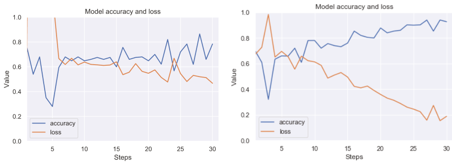
Figure 12. Exemplary learning effect before (left side) and after using our technique (right side). Result for RIYADH dataset. Class ok (without artefacts) vs. class er (with strong artefacts). The line graphs shows accuracy (blue) and loss (orange) for 15 epochs (30 steps from batch). Although the image dataset is relatively small for Convolutional Neural Network (CNN), there can be observed a good trend in increasing accuracy, while minimizing loss.
