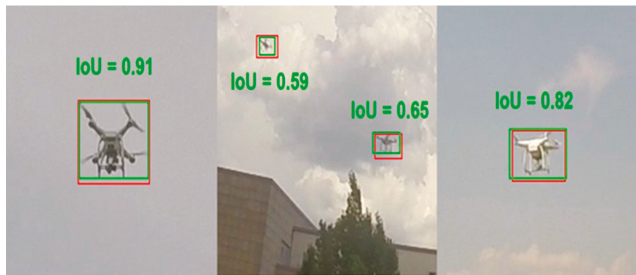
Figure 8. Qualitative results of our detector. Green bounding boxes are ground truth bounding boxes. Red bounding boxes are the results of applying our detector.
