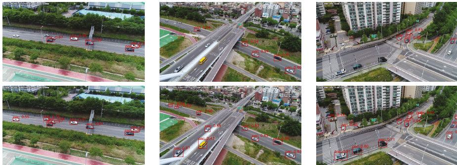
Figure 14. Experiment results of DRFBNet300 trained on UAV-cars dataset ( top ) before and ( bottom ) after applying SIP.
