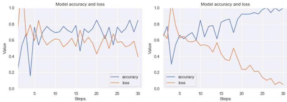
Figure 17. Exemplary learning effect before (left side) and after using our technique (right side). Result for MOSCOW dataset. Class 0 (without artefacts) vs. class I (with weak artefacts). The line graphs shows accuracy (blue) and loss (orange) for 15 epochs (30 steps from batch). Although the image dataset is relatively small for CNN, there can be observed a good trend in increasing accuracy, while minimizing loss.
