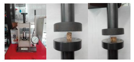
Figure 4. Axial compressive test.
