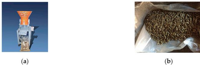
**Figure 3.** N-Pico pelletizer (a) and pelletized rice straw (RS) (b).
