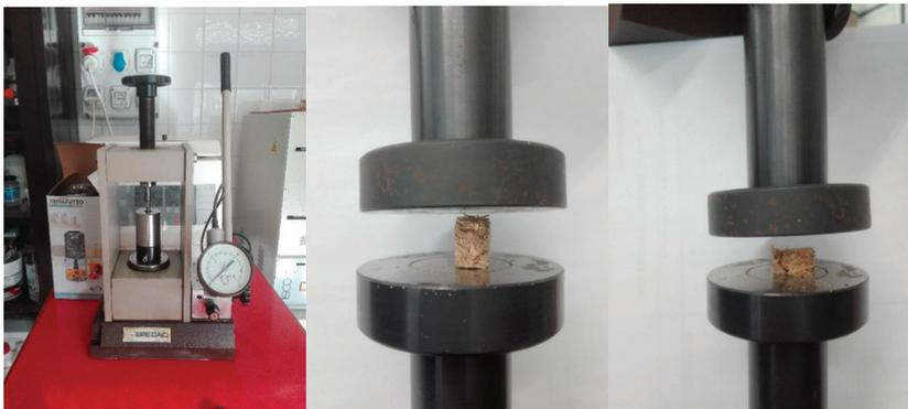
Figure 4. Axial compressive test.
