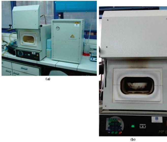
**Figure 1.** Experimental setup of the torrefaction process: (a) Nuve Muffle Furnace (Internal dimensions: 210W × 300D × 110Hmm) equipped with electric heating and a nitrogen generator that uses molecular sieves and (b) barley straw in a ceramic crucible placed in the cold furnace.
