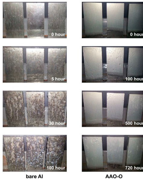
Figure 6. Results of salt spray test for bare aluminum and AAO-O (oil impregnation on anodic aluminum oxide) surfaces.
