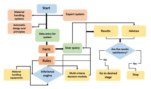
Figure 2. Configuration of modules in the material handling equipment selection process.
