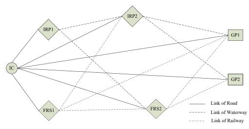
**Figure 1.** The proposed port-hinterland intermodal transportation network. FRS, freight rail station; IRP, inland river port; IC, inland city; GP, gateway seaport.
