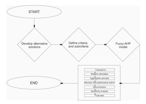
Figure 2. Multiple-criteria decision-making (MCDM) model for the selection of optimal underground mining method.
