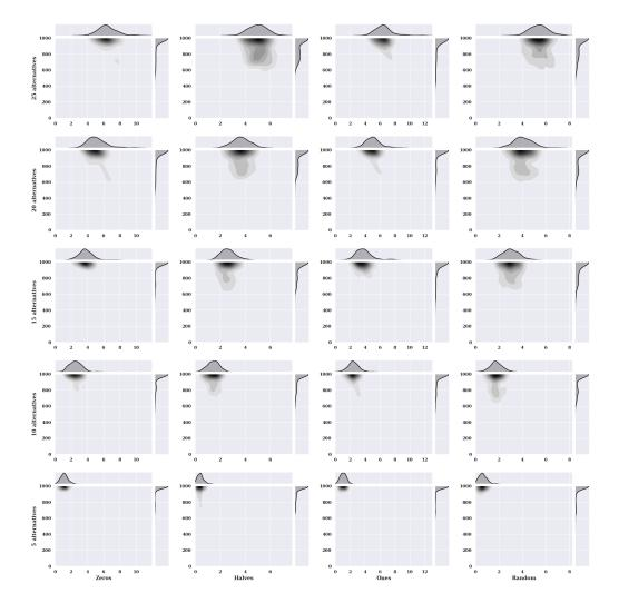
**Figure 7.** The value of the target function depending on the number of iterations, the number of alternatives, and initial conditions (method: SA; criteria variant: dynamic; model: not existing).
