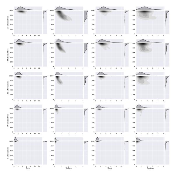
**Figure 8.** The value of the target function depending on the number of iterations, the number of alternatives, and initial conditions (method: SA; criteria variant: static; model: existing).
