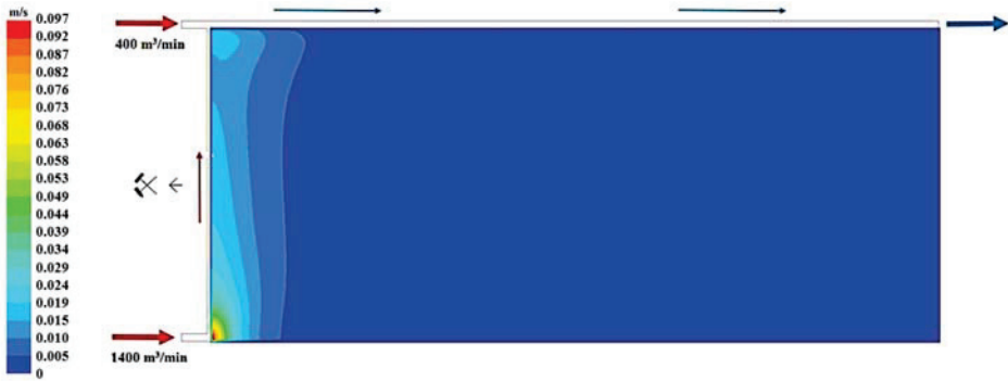
Figure 10. The distribution of the air speed flowing through the goaves with caving at a distance of 7.0 m from the floor of the exploited seam.
