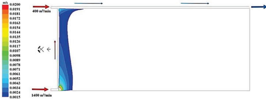
Figure 5. The distribution of the air speed within the range from 0.02 m/s to 0.0015 m/s flowing through the goaves with caving at a distance of 0.5 m from the floor of the exploited seam.
