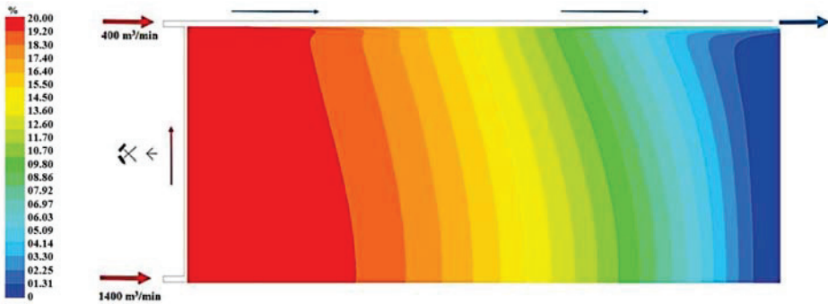
Figure 24. The distribution of oxygen concentration in the air flowing through the goaves with caving at a distance of 2.0 m from the floor of the exploited seam.
