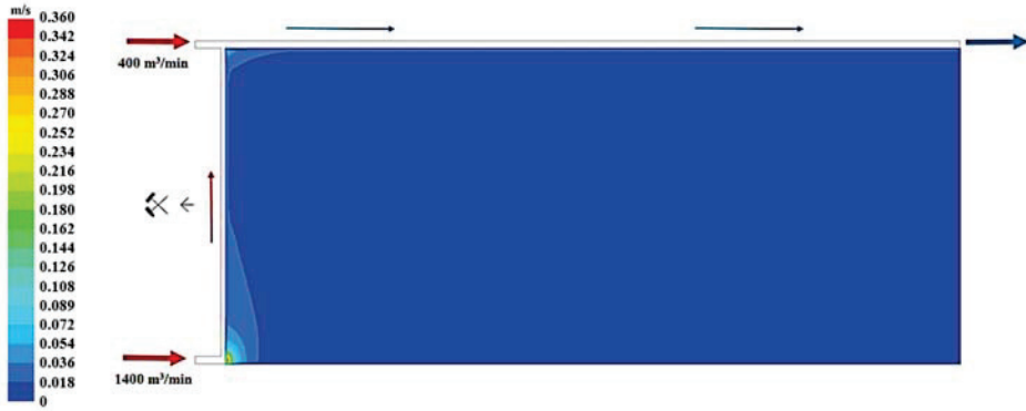
Figure 7. The distribution of the air speed flowing through the goaves with caving at a distance of 2.0 m from the floor of the exploited seam.
