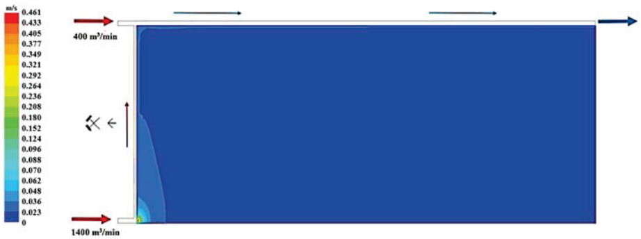
Figure 22. The distribution of the air speed flowing through the goaves with caving at a distance of 2.0 m from the floor of the exploited seam.
