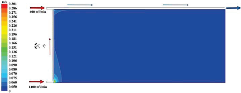
Figure 4. The distribution of the air speed flowing through the goaves with caving at a distance of 0.5 m from the floor of the exploited seam.
