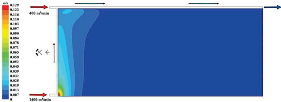
Figure 25. The distribution of the air speed flowing through the goaves with caving at a distance of 7.0 m from the floor of the exploited seam.
