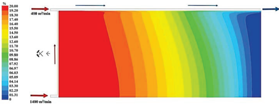
Figure 21. The distribution of oxygen concentration in the air flowing through the goaves with caving at a distance of 0.5 m from the floor of the exploited seam.
