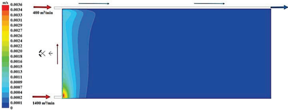
Figure 13. The distribution of the air speed flowing through the goaves with caving at a distance of 10.5 m from the floor of the exploited seam.
