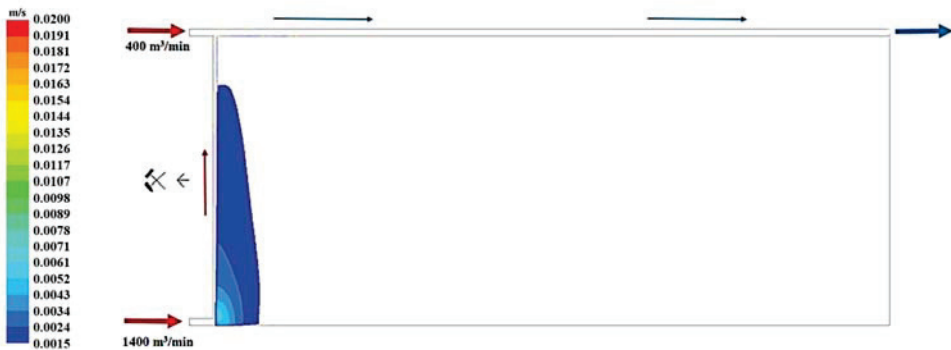
Figure 29. The distribution of the air speed within the range from 0.02 m/s to 0.0015 m/s flowing through the goaves with caving at a distance of 10.5 m from the floor of the exploited seam.
