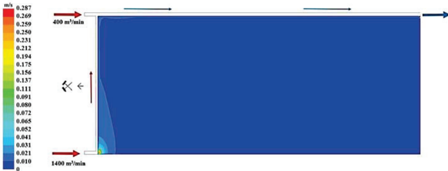
Figure 19. The distribution of the air speed flowing through the goaves with caving at a distance of 0.5 m from the floor of the exploited seam.
