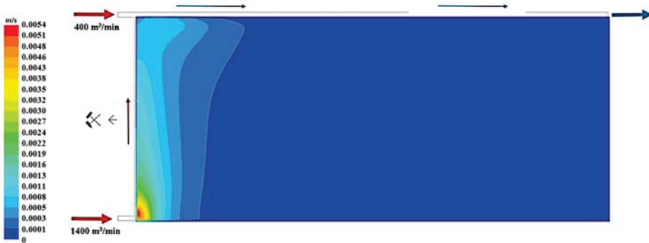
Figure 28. The distribution of the air speed flowing through the goaves with caving at a distance of 10.5 m from the floor of the exploited seam.
