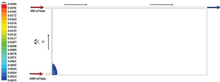
Figure 14. The distribution of the air speed within the range from 0.02 m/s to 0.0015 m/s flowing through the goaves with caving at a distance of 10.5 m from the floor of the exploited seam.
