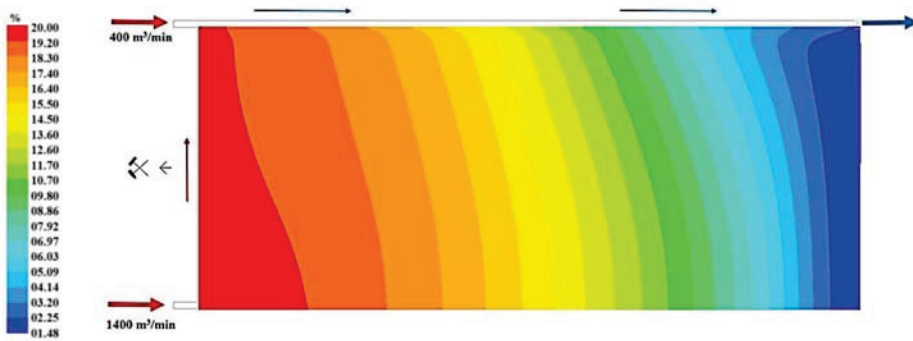
Figure 30. The distribution of oxygen concentration in the air flowing through the goaves with caving at a distance of 10.5 m from the floor of the exploited seam.
