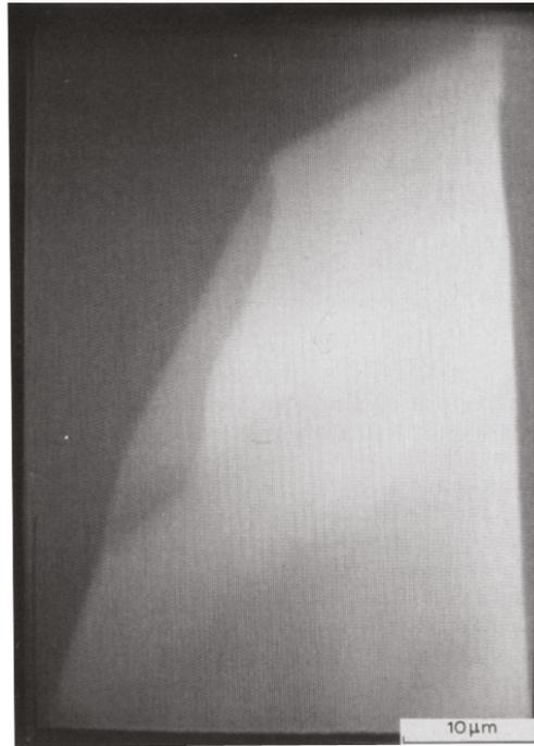
**Figure 3.** A bulge formed at a grain boundary of  $\beta$ -Ti6Al-2V-6Zr alloy during rapid heating (photoemission electron microscope PEEM).
