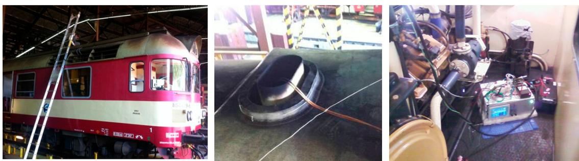
**Figure 5.** Series 854 diesel-hydraulic railcar tests: installation of the sampling line (left); sampling probe (middle); and portable emissions monitoring system (right).
