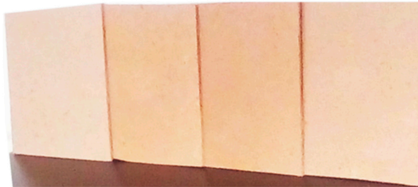
Figure 1. High-density fiberboards from industrial hardwood fibers bonded with UF resin and ammonium lignosulfonate; 910 \text{ kg}\cdot\text{m}^{-3} target density, 6 mm thickness and three addition levels of ammonium lignosulfonate (6%, 8%, 10%).
