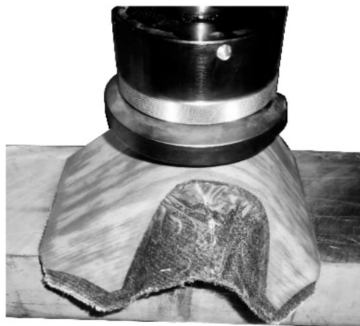
Figure 5. Bending test for 3D molded plywood samples.
