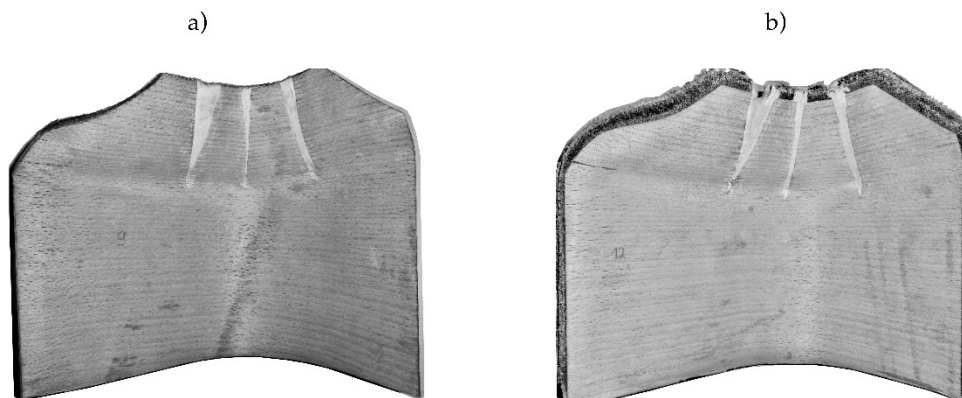
Figure 4. Relief cut of specimens (a) reference, (b) with flax fiber reinforcement.
