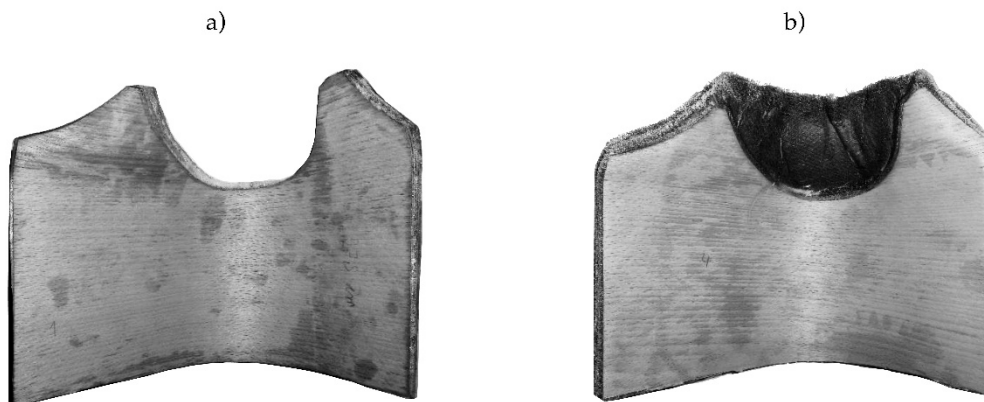
Figure 3. Cut-out of specimens (a) reference, (b) with flax fiber reinforcement.
